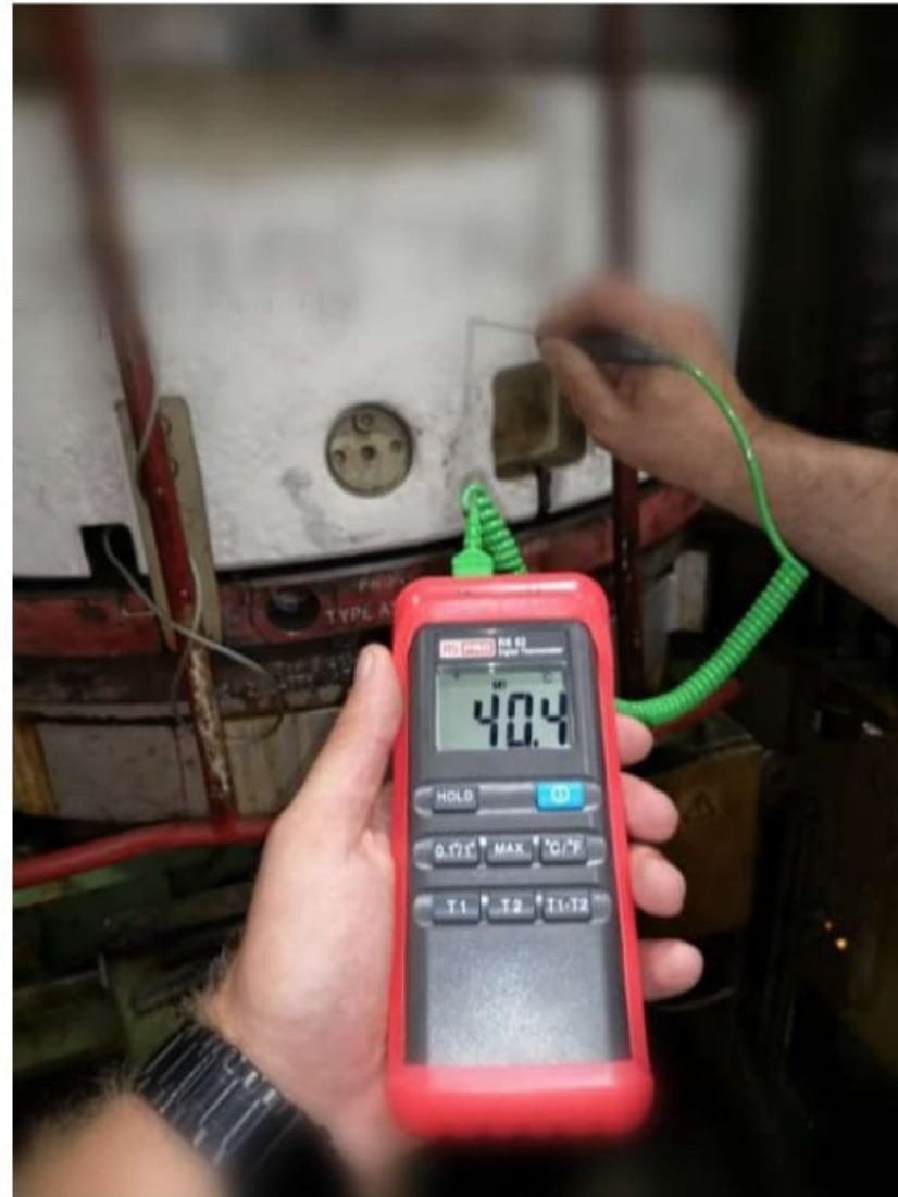
Measuring no. 3: Surface temperature insulated by PS Coat: 40,4 °C
